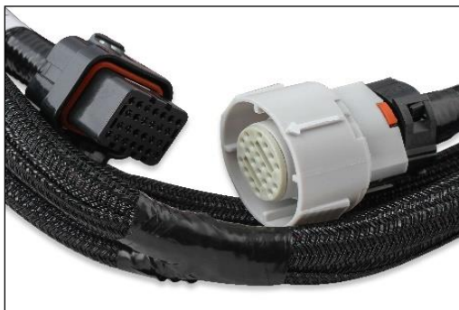
Figure 32 - Transmission & ECU Connector
