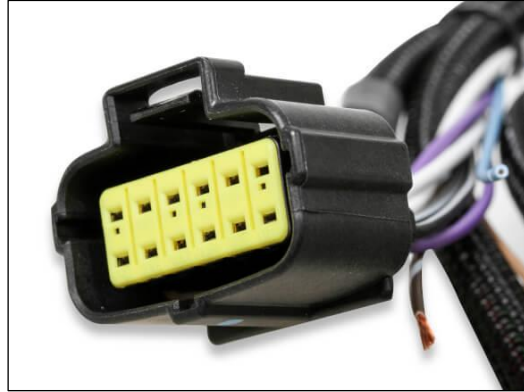
Figure 35 - Main Transmission Connector 4R70W/4R75W 98+
