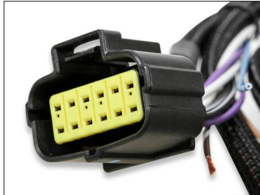
Figure 35 - Main Transmission Connector 4R70W/4R75W 98+
