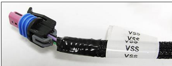
Figure 30 - Vehicle Speed Sensor
