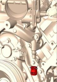
If ONLY installing the Holley ADD-ON power steering to wet sump applications, install the supplied red cap to the water pump barb. After installation, rotate the cap until the text is forward. See APPENDIX for alternate oil cooler plumbing.
