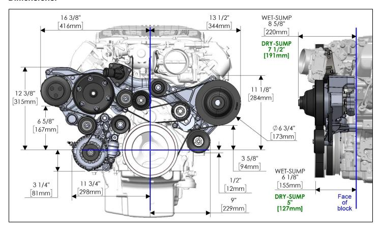
**IMPORTANT NOTE IF PAINTING COMPONENTS:** The alternator and A/C compressor ground through the bracketing. If painting or coating the alternator bracket or water pump manifold, the mating surfaces must all be bare metal allowing a ground path from the accessories' mounting feet to the engine block and ultimately the negative terminal on the battery.
