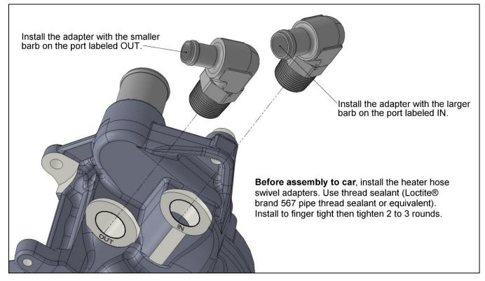
**HELPFUL HINT:** The below assembly order is optimized for explanation and the average application. For your application, determine if it is easier to assemble before or after the water pump manifold is mounted to the engine. Keep in mind adding components before mounting increases overall size and weight and will require an additional person when mounting to the engine. Torqueing of the component's bolts may be easier after mounting.
