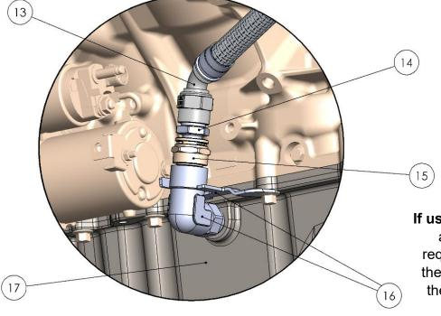
Route oil drain back hose (12) safely away from heat sources and any exhaust components.
