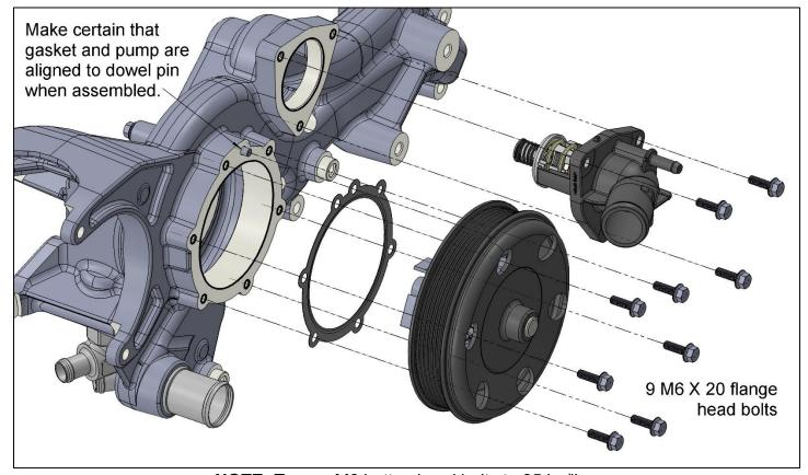
NOTE: Torque M6 button head bolts to 85 in./lbs.
