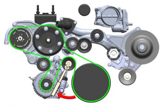
**NOTE:** For easy belt installation, route onto all pulleys leaving one smooth idler pulley for last. It is best if this last smooth pulley is not the tensioner pulley.
