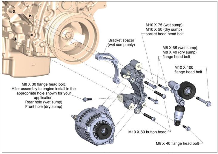
NOTE: Torque M8 bolts to 18 ft./lbs. Torque M10 bolts to 36 ft./lbs.
