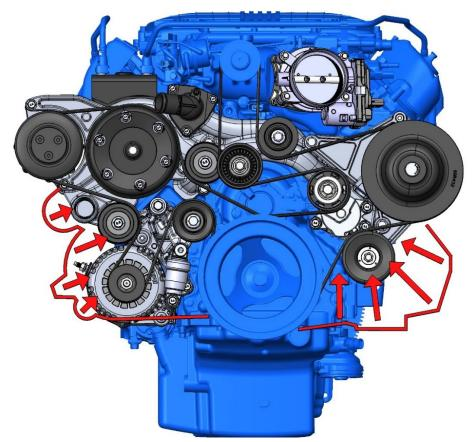
Not only does the Holley's accessory drive add a reliable power steering solution, it also pulls in accessories tighter than other drives allowing clearance for steering boxes, suspension, and frame rails in swap applications.
