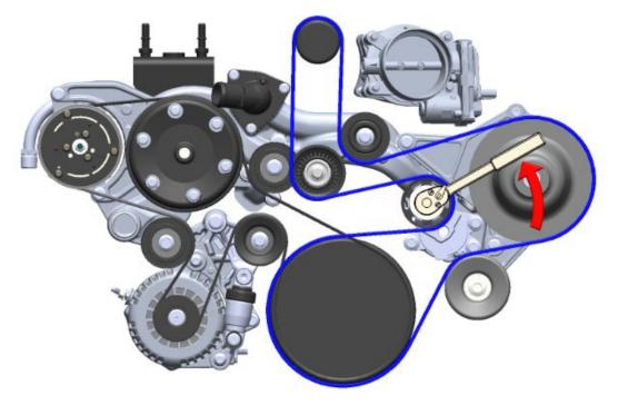
SECOND: Install the supercharger belt as shown below
