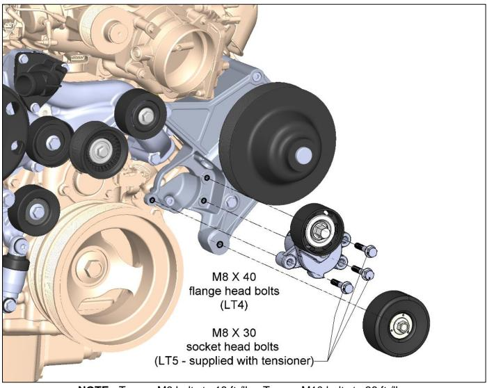
NOTE: Torque M8 bolts to 18 ft./lbs. Torque M10 bolts to 36 ft./lbs.
