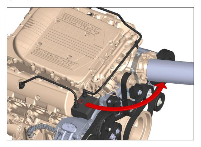
The separator tank vent plumbing is custom as the intake tube in swap applications vary. Earl's 90 degree 1/2" NPT to male -6 AN adapter P/N AT982268ERL can be used to adapt the tank vent to standard AN.
