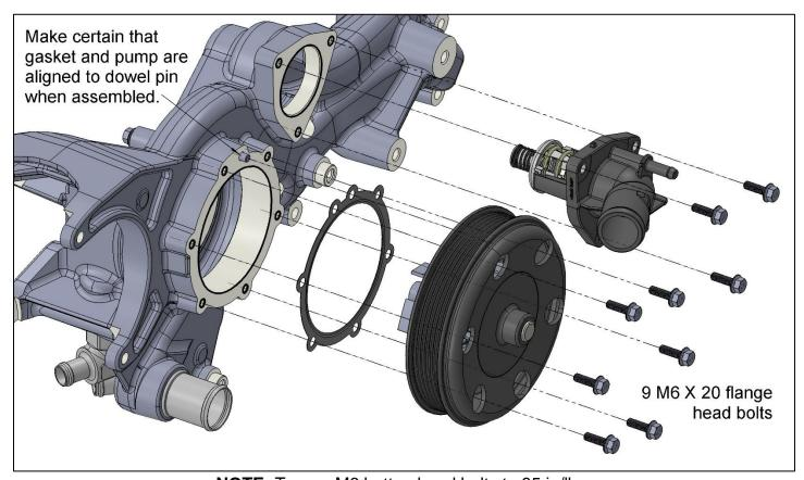
**NOTE:** Torque M6 button head bolts to 85 in/lbs.
