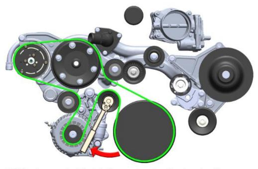
**NOTE:** for easy belt installation, route onto all pulleys leaving one smooth idler pulley for last. It is best if this last smooth pulley is not the tensioner pulley.
