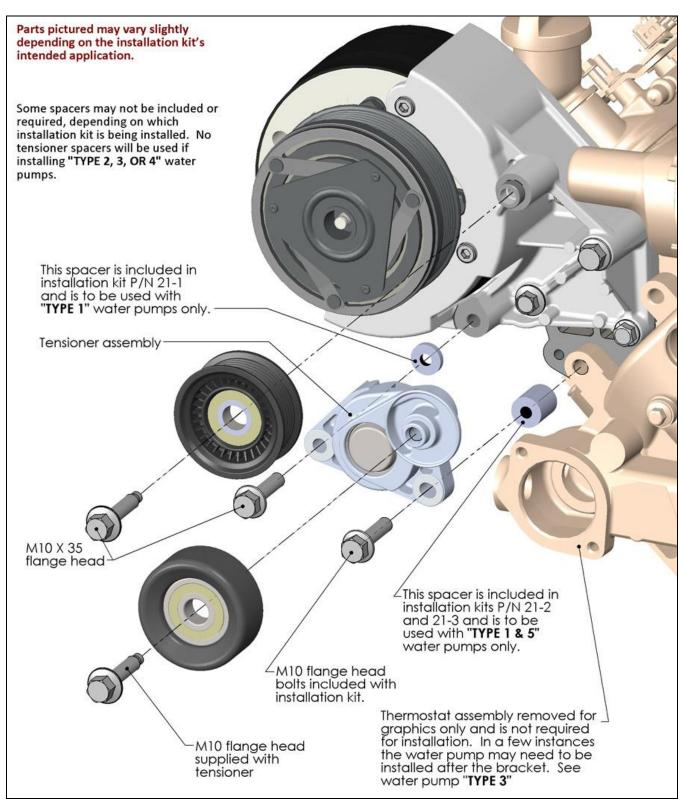
NOTE: Torque M8 bolts to 18 ft./lbs. and M10 bolts to 36 ft./lbs.
