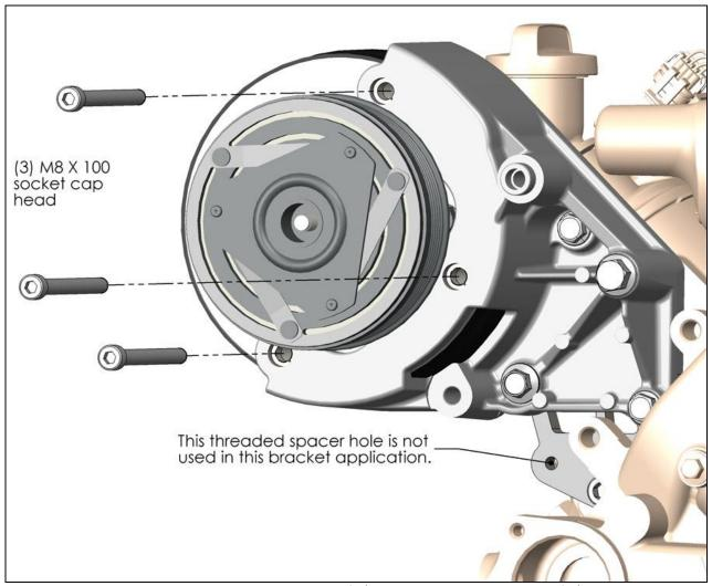
NOTE: Torque M8 bolts to 18 ft./lbs. and M10 bolts to 36 ft./lbs.
