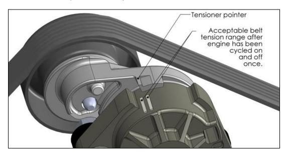
**NOTE:** If you are NOT using this system with P/N 20-143, you will have to measure to find the correct belt length.
