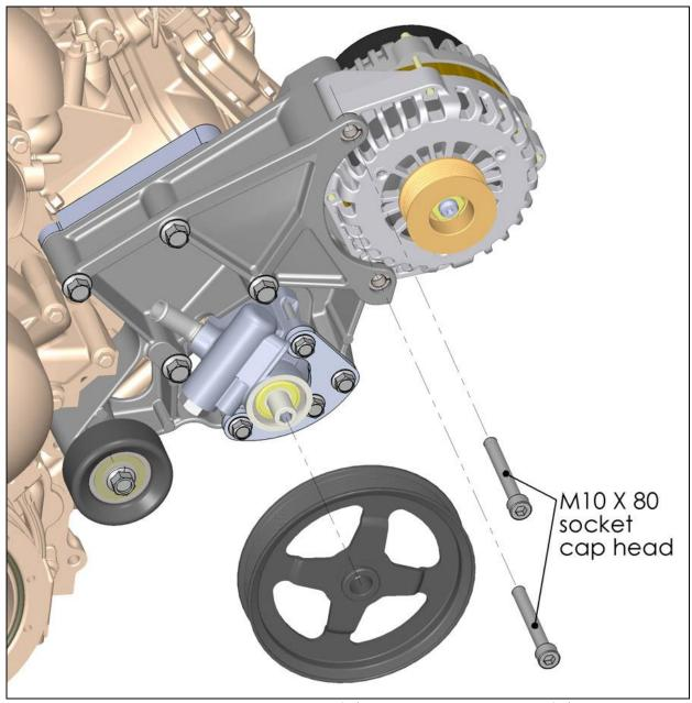
**NOTE:** Torque M8 bolts to 18 ft./lbs. and M10 bolts to 36 ft./lbs.
