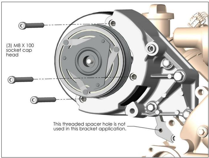
NOTE: Torque M8 bolts to 18 ft./lbs. and M10 bolts to 36 ft./lbs.
