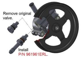
NOTE: If using AN fittings on the pressure line, Holley P/N 961961ERL AN extension/adapter is required.
