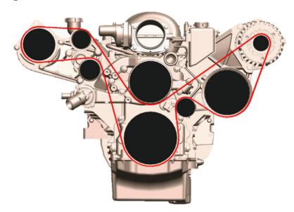
**HELPFUL HINT:** When installing the belt, route around all the pulleys except the water pump pulley. While fully rotating the tensioner arm, slip the belt on the smooth water pump pulley last.
