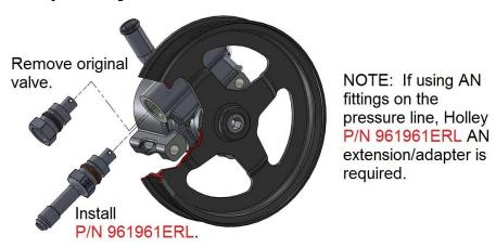
There are several pulleys that will fit the pump, but some do not have the correct belt alignment for this application. See applicable service manual for pulley installation procedures.
