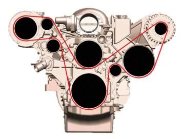
**HELPFUL HINT:** When installing the belt, route around all the pulleys except the water pump pulley. While fully rotating the tensioner arm, slip the belt on the smooth water pump pulley last.
