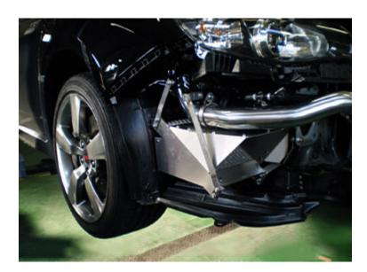
GRB bumper has a small opening; therefore the <u>air intake</u> is also limited. To get enough air for cooling, HKS GRB Oil Cooler has many features for the best condition for engine.
