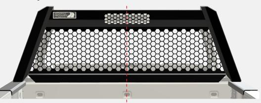
Slide Headache Rack Feet inward or outward to desired fit.
