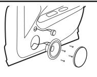
C Tweeter mounting There are two primary ways the tweeter can be mounted. Surface and Flush mounting. The flush mount configuration is shown here.
