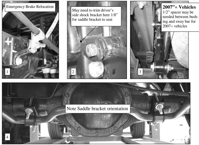
BEFORE INSTALLATION OF SWAY BAR ASSEMBLY, RELOCATE EMERGENCY BRAKE CABLE USING SUPPLIED BRACKET AND 5/16 BOLT AS SHOWN IN PHOTO (1).
