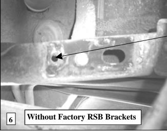
Vehicles w/o factory RSB brackets. Enlarge this hole using 1/2" Drill bit. This hole will be used to attach the clevis to the frame using the supplied 1/2" bolt, locknut, and washer.
