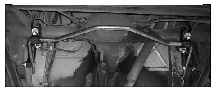
Washer between frame bracket and bushing. Apply red loc-tite to bolt and torque to 40 ft-lb
