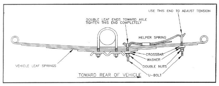
**NOTICE: Do Not** attempt to install this unit on any vehicle with composite (plastic) leaf springs, this includes certain years of Chevy Astro, GMC Safari Vans, Ford Ranger, and Mazda B3000, B4000 Pickups. Damage to the composite spring can result.
