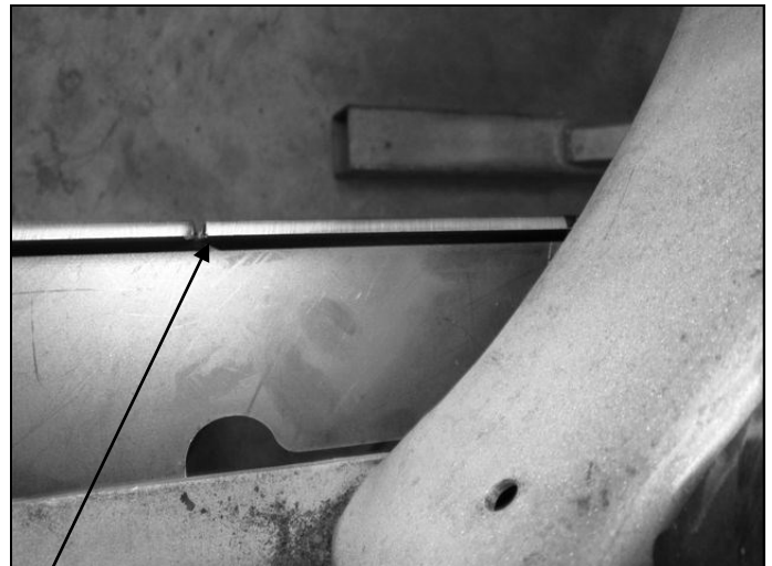
Flex end of forward plate upward to close gap Cut in vertical flange will allow plate to be flexed. The cut can be welded and ground smooth after fitment and tacking in place.
