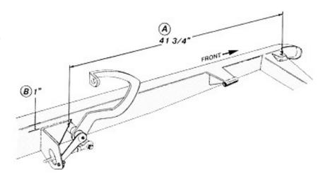
PLEASE NOTE: The above dimensions place the pedal assembly in the optimum position for use with our Model 'A' chassis and components. Minor changes may be required to find the best position on your chassis.
