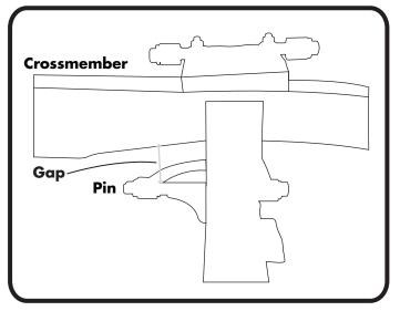
2 Using template cut plate to fit
