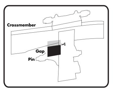
3 Weld into place between the pin and crossmember
