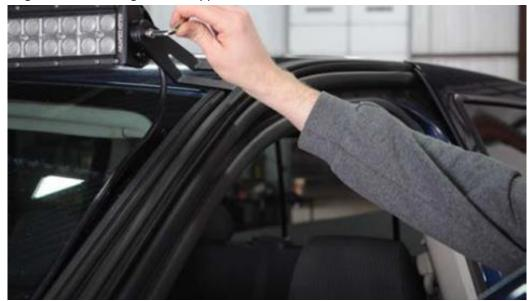
8. Adjustments to the light bar can now be made to achieve the desired angle and then tighten bolts down.
