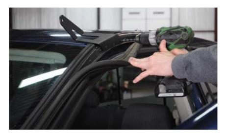
5. With a rivet gun, use the supplied 3/16" rivets to secure the mount to the cab.
