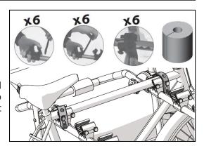
D. Use the extra strap to secure bike tires/frames to the bike rack and prevent the bikes from swaying while on the road.
