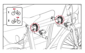
5. Load bikes alternatively and secure them by using rubber straps.
