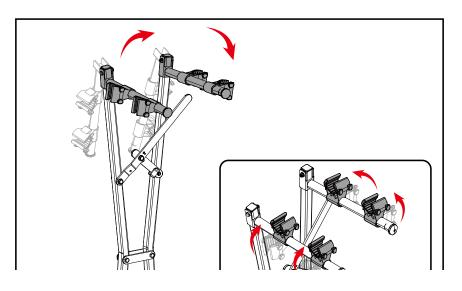
spread the top of the tubes away from each other so they nest on the 2 x 2 insert tube.
