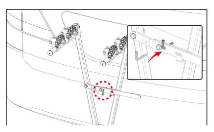
3. Insert the security pin, and turn 180 degrees. Then insert the bridge pin through the small hole in the pin.
