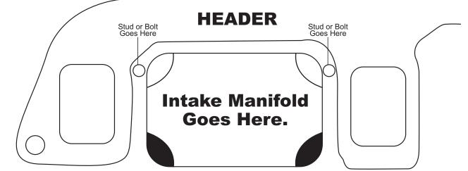
If spacer is to long it may need to be cut to adjust difference in height between intake manifold and hedder head flange. (If minimal amount of spacer remains, may need to use mill washer, cut 1/3 washer away to use as spacer.)
