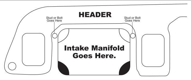
If spacer is to long it may need to be cut to adjust difference in height between intake manifold and hedder head flange. (If minimal amount of spacer remains, may need to use mill washer, cut 1/3 washer away to use as spacer.)
