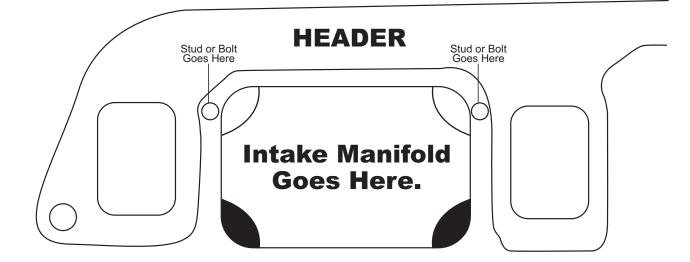
If spacer is to long it may need to be cut to adjust difference in height between intake manifold and hedder head flange. (If minimal amount of spacer remains, may need to use mill washer, cut 1/3 washer away to use as spacer.)
