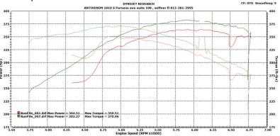
After the I-M Shield was installed, the LS1 cranked out 382 horsepower and 370 lb-ft of torque. That's a gain of 18 and 20, respectively.
