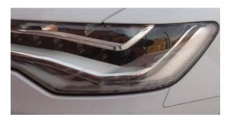
the air vents, humidity is sucked into the headlight from the outside. So, when you turn off your headlights after hours of driving, low pressure inside the headlight draws humid air in, thus the fogging of the lens occurs.
