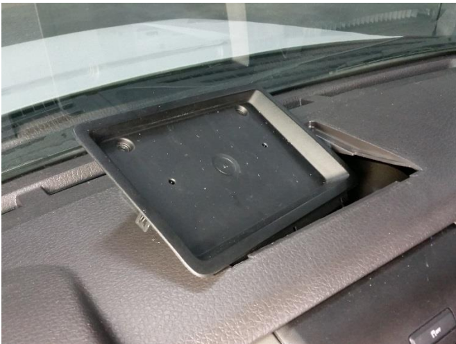
Remove two (2) 7mm head fasteners. Set aside factory change tray. It will not be reused.
