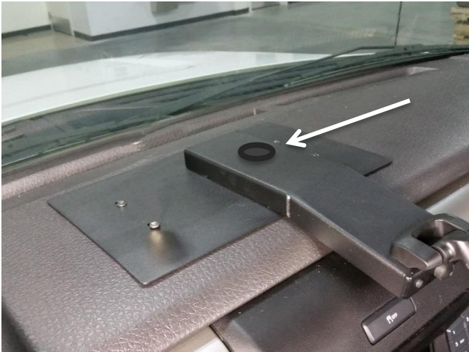
Install dash mount bracket and run harnesses through center of support.
