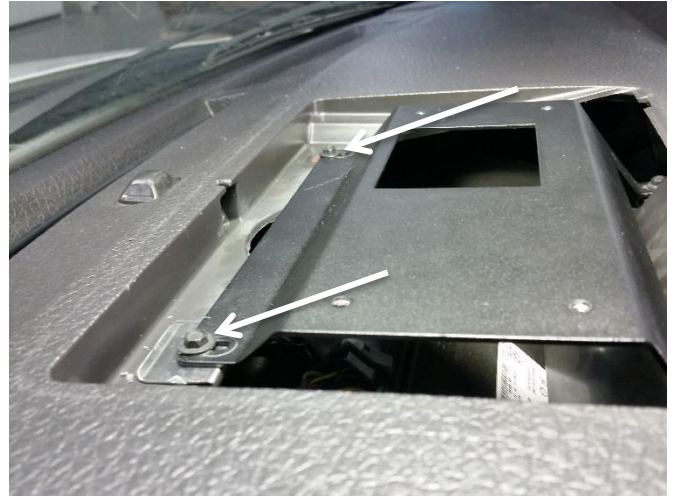
Install forward fasteners using previously removed hardware from change tray.
