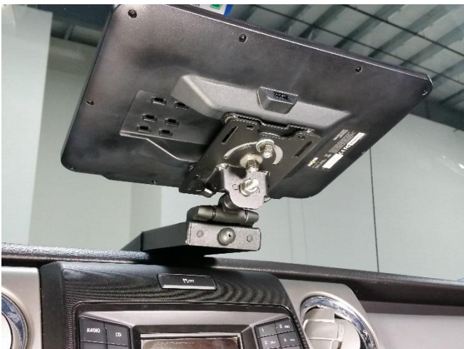
Attach bracket with display to the tilt swivel hinge with M8 hex nut and lock washer. Tighten nut and attach vinyl cap on M8 bolt threads.
