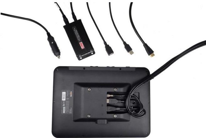
Connect harnesses to the back of the TSD-101 display. It is important to also double wire tie the harnesses to provide sturdy strain relief for the plugs. USB connection from remote Docking station must plug into USB plug closest to front of display.
