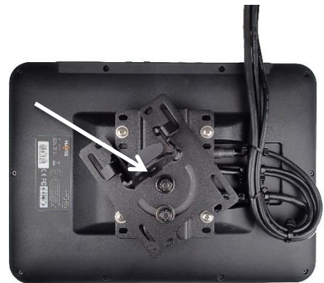
Attach pivot / display mount bracket to display with M4 x 0.7 x 10mm Phillips head machine screws, lock washers and flat washers. Display mount hardware is included with TSD-101 hardware kit
