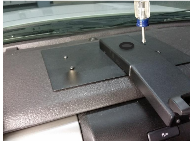
Install and tightened four (4) 10-32 x 1/2" machine screws and #10 washers.
