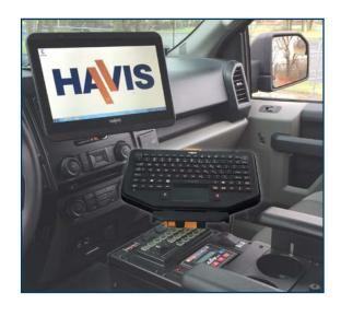
The System includes the Havis Rugged Keyboard (KB-101) and Keyboard Mount (C-KBM-201). Featuring red monochrome backlit illumination to reduce eye strain, the IP65 rated keyboard rests securely in the patent pending mount allowing ease of use and adjustment.
