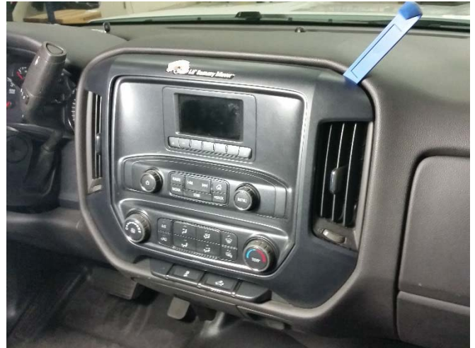
Remove dash panel by gently prying along edges with a panel removal tool.
