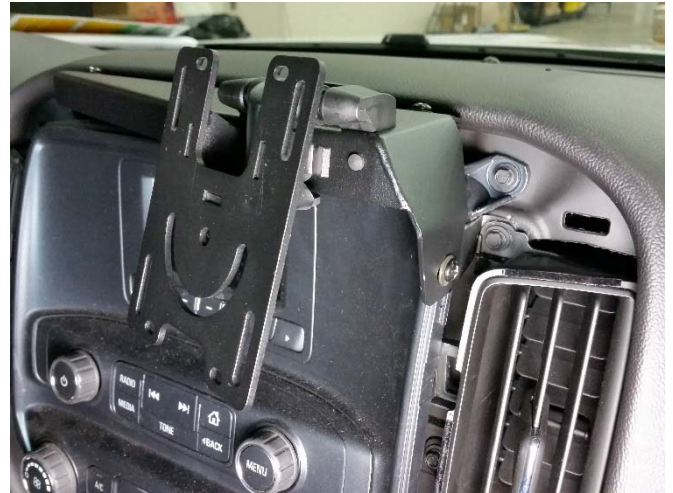
Loosely attach main dash mount bracket and ensure fitment.
