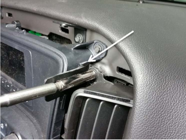
Install passenger side mounting tab using previously removed hardware.
