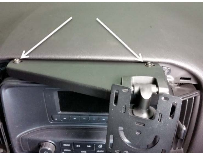
Re-install dash trim and place main dash mount onto the tabs.
