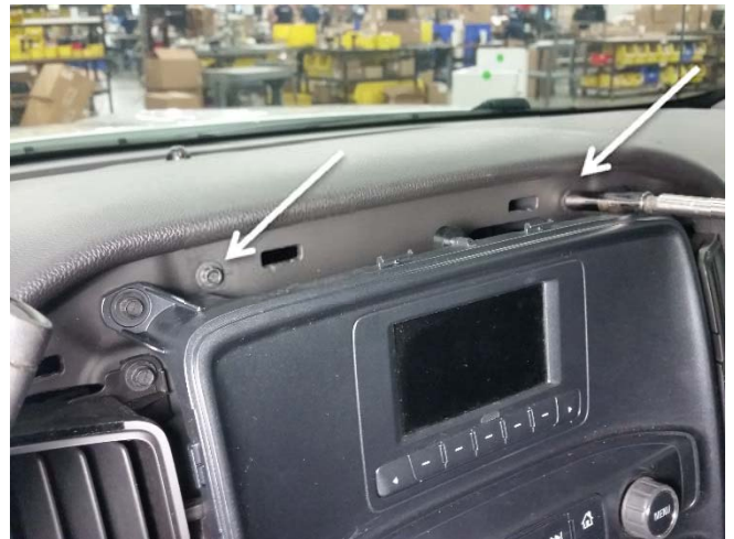
Remove fasteners above radio display (7 mm socket)
