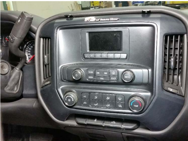
Remove dash mount bracket and gently place trim back on dash.
