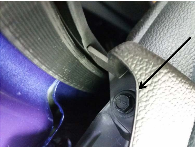
Remove 7mm head fasteners located at base of "A" pillar.
