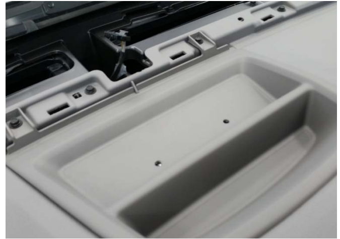
Re-install OEM tray assembly and verify holes line up to the upper mounting bracket. Drill holes slightly larger in plastic for additional clearance if necessary.
