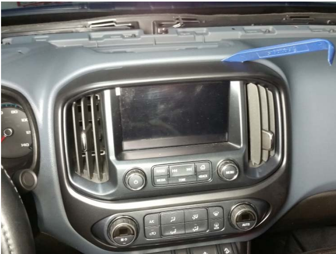
Remove trim bezel around display and HVAC controls by gently prying along the frame.
