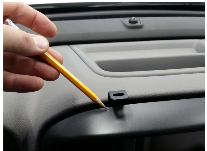
Hold radio trim bezel up to the dash and mark location of brackets. Notch material as needed to allow trim to properly snap back into place.
