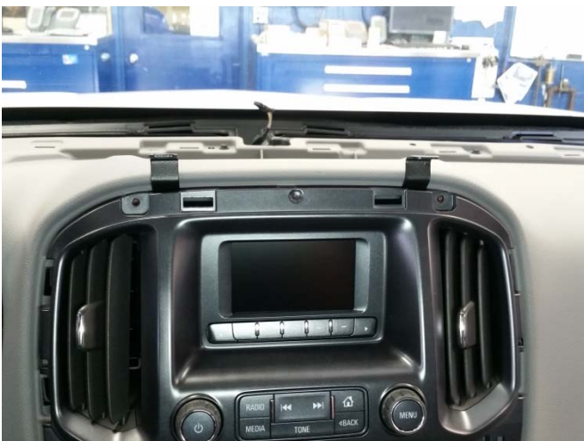
Re-install display and HVAC control.
