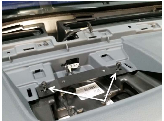
Use OEM hardware and attach upper mounting bracket # CM008207 to OEM inserts.
