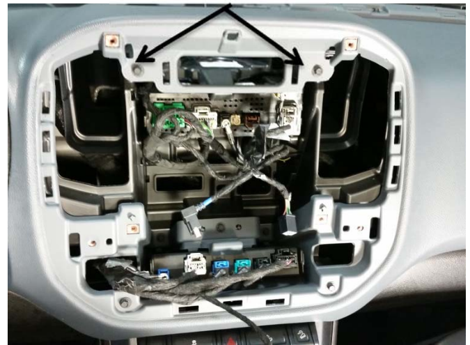
With display removed, attach the mounting brackets # CM008154 to existing upper OEM fasteners.
