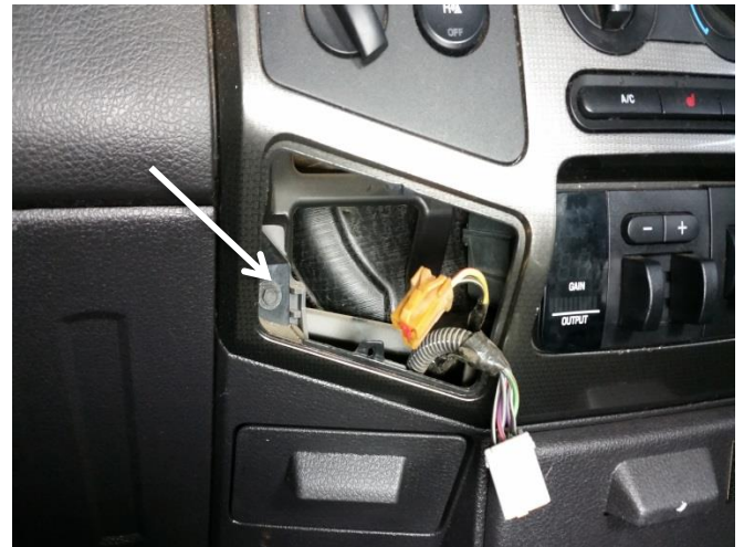
Remove panel containing OEM 12v socket. Remove fastener. (7 mm socket)
