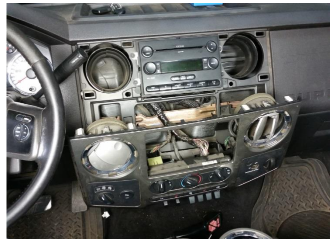
Remove dash panel by gently prying along edges with a panel removal tool.
