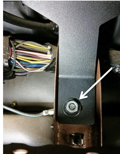
Use M6 nut and 1/4" washer to attach bracket to existing threaded stud.
