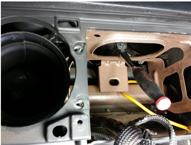
Tighten hardware. (10mm socket)
