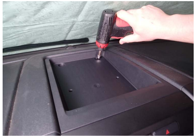
Remove two (2) fasteners from the forward section of the tray Note: If equipped with center channel speaker, simply pop up grill to access screws.
