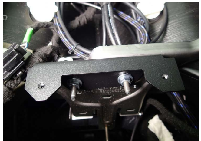
Attach lower bottom support bracket to OEM M6 studs using two (2) M6 nuts. Note: Vehicle with Sync 3 option will have a module that shares these mount studs.
