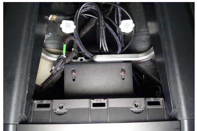
Install upper bottom support bracket onto lower bottom support bracket using two (2) 8-32 x 5/8" bolts and washers.
