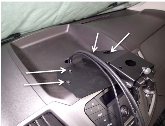
Install main mounting bracket onto the tray and secure to the lower mounting base using four (4) 8-32 x 5/8" machines screws.
