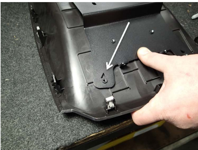
Line up triangle cutouts in the bracket to the seams in the tray.
