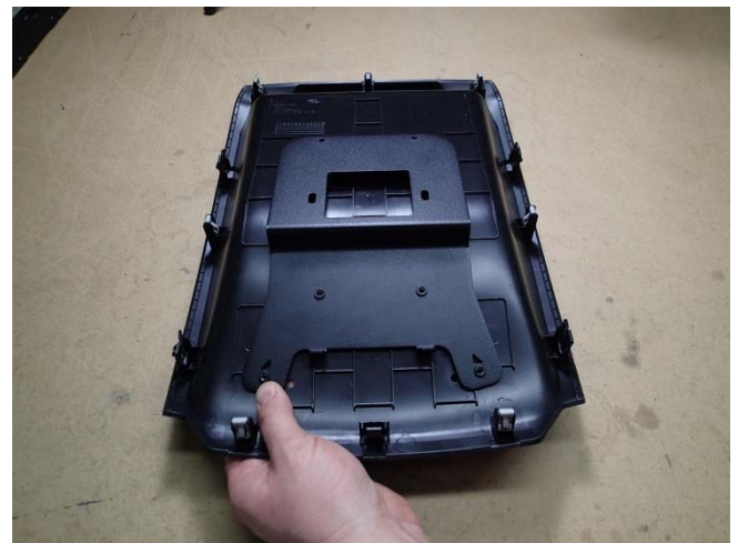
Place the main dash mount base to the bottom of the previously removed tray
