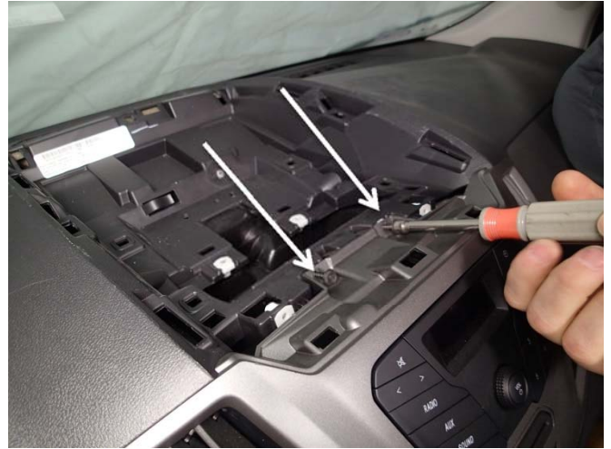
Remove factory hardware from top of radio housing using. (7mm socket)
