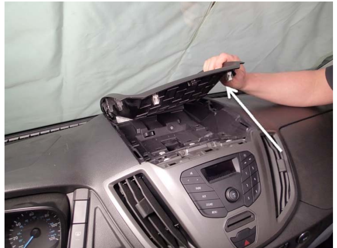
Carefully remove top pocket by gently prying along seams
