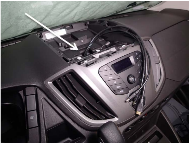
Running computer wires through the dash is recommended at this time
