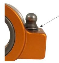
The rocker adjusters are a 7/16-20 screw with a 5/16 ball. You have to use pushrods with a 5/16 cup end. When setting pushrod length have no more than 2 and no less then 0 threads showing on the bottom side of the rocker, between the ball and rocker body. This is to make sure the pushrod contact point and rocker geometry are correct.
