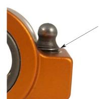
The rocker adjusters are a 7/16-20 screw with a 5/16 ball. You have to use pushrods with a 5/16 cup end. When setting pushrod length have no more than 2 and no less then 0 threads showing on the bottom side of the rocker, between the ball and rocker body. This is to make sure the pushrod contact point and rocker geometry are correct.
