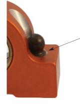
The rocker adjusters are a 7/16-20 screw with a 3/8 ball. You have to use pushrods with a 3/8 cup end. When setting pushrod length have no more than 2 and no less then 0 threads showing on the bottom side of the rocker, between the ball and rocker body. This is to make sure the pushrod contact point and rocker geometry are correct.
