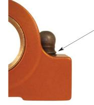
The rocker adjusters are a 7/16-20 screw with a 3/8 ball. You have to use pushrods with a 3/8 cup end. When setting pushrod length have no more than 2 and no less then 0 threads showing on the bottom side of the rocker, between the ball and rocker body. This is to make sure the pushrod contact point and rocker geometry are correct.
