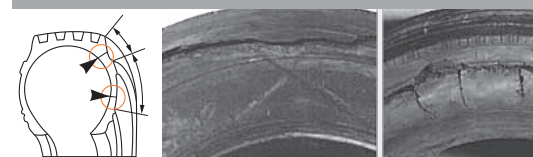
Sidewall damage due to run flat or severe under inflation
