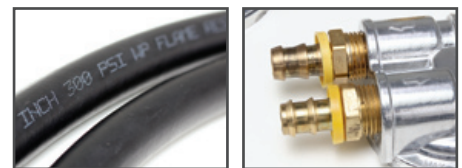
CAST relocation kits include 30" high-temp/pressure Oil Lines
