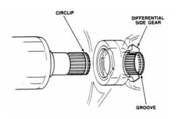
1. When installing the new axle be sure the cir-clip on the inner joint stub locks into the transmission.
