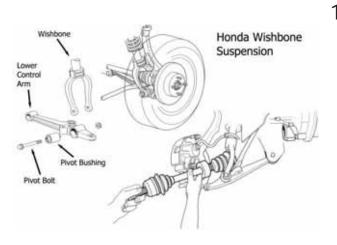
11. On Honda's, with wishbone suspension, the pivot bolt has a tendency to seize to the inner sleeve of the pivot bushing. Instead of removing the pivot bolt and risk damaging the bushing. Disassemble the inner joint and remove the axle in two separate pieces.
