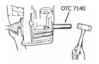
9. On some Escort & Lynx models you will need to remove the right hand CV shaft before removing the left hand shaft. The Ford differential rotator tool can be used to remove the left hand shaft. If both shafts are removed leave the rotator tool in the differential so the side gears will stay aligned.
