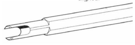
10. Various Renault models use two roll pins to hold the inner joint on to the transmission stub. One roll pin is inside of the other. Be sure to remove both of the roll pins before attempting to remove the axle.
