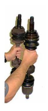
1. Before installing the new axle match it to the old unit. Check the over all compressed length by bottoming both inboard joints on something hard like a cement floor.
