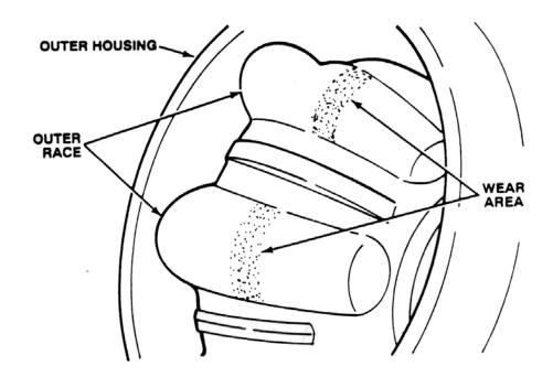
The only way to properly repair a joint with this type of indention is to replace the worn components or machine them to accept an over-sized ball.
