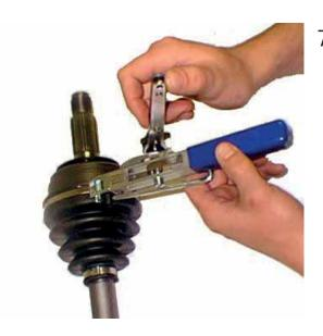
7. The clamps supplied with this kit are universal-type. Wrap the clamp around the boot and insert the end of the clamp into the clamp tool. Ratchet the clamp tool till the clamp is tight. Be careful not to over tighten the clamp so it cuts the boot. Cut the band with the clamp tool and fold the end back between the tabs. Fold the tabs over to lock the end in place.
