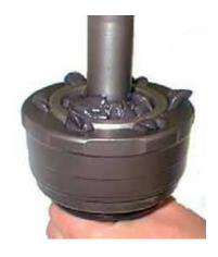
4. Install the center shaft into the race of the outer joint. The pressure will force the grease out through the balls. The grease that squeezes out through the balls should be cleaned off with a rag.
