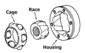
3. The cross groove style joint can be assembled two different ways. The correct way is to align the grooves in the race to cross the grooves in the housing so they make an X pattern. If the joint is not assembled properly it will not plunge and move freely.
