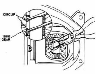
5. The Chrysler vehicles listed below use a cir-clip to retain the axles into the transmission. This clip must be compressed before the axles can be removed from the transmission. Remove the differential inspection cover, compress the tangs of the clip with needle nose pliers, and remove the axle from the transmission.
