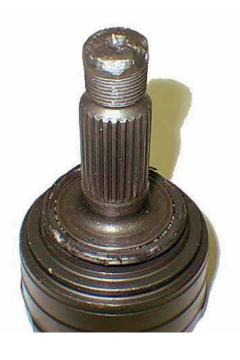
4. Do not use a hammer to drive the C.V. Joint out of the hub. This will damage the joint and the core will have no value.
