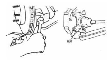
3. After pushing the outer joint through the hub, install the ball joint and nut or bolt.
