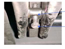
TORSION BAR ADJUSTER BOLT RETAINING PLATE.
