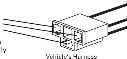
2. If your vehicle wiring matches the H4 wiring, you can set the adapter harness aside and plug your new Grote LED headlamps directly into your vehicle's H4 connector.
