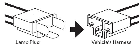
3. For all other configurations snap each wire of the adapter harness (A) into the proper location in the plastic adapter block (B) to match your vehicle wiring. See the wire color code of the adapter Harness below:
