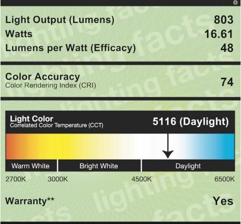
All results, except LED Lumen Maintenance, are according to IESNA LM-79-2008: Approved Method for the Electrical and Photometric Testing of Solid-State Lighting. The U.S. Department of Energy (DOE) verifies product test data and results.
